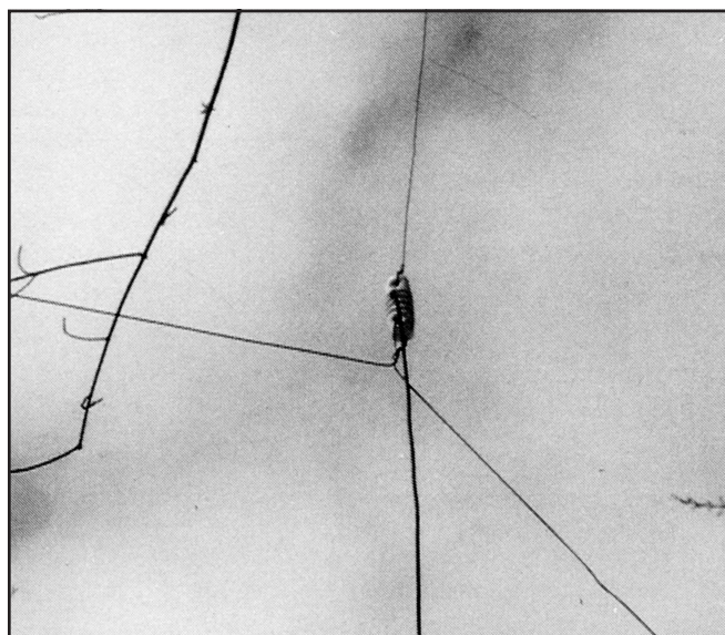
Fig 4 —The feed point of the tree-mounted groundplane antenna. The opposite ends of the two radial wires may be connected to stakes or other convenient anchor points.
