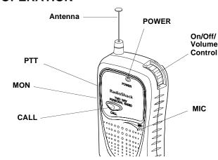
Antenna — extend when receiving and transmitting.
