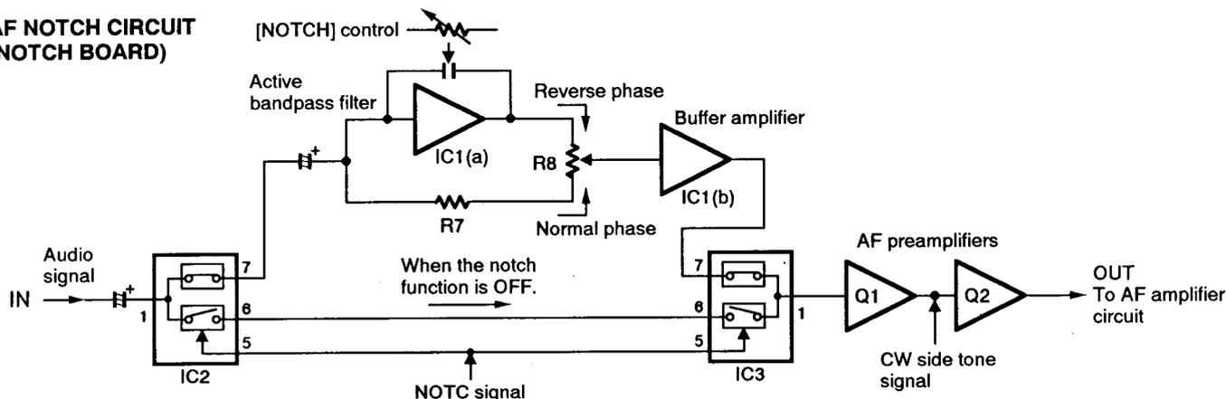
The signal is then applied to an active bandpass filter (IC1a), which has very narrow width characteristics, to pick up the interference frequency in reverse phase. The resulting signal is mixed with the original signal at R8 to obtain approx. 20 dB attenuation of the interference frequency components.
