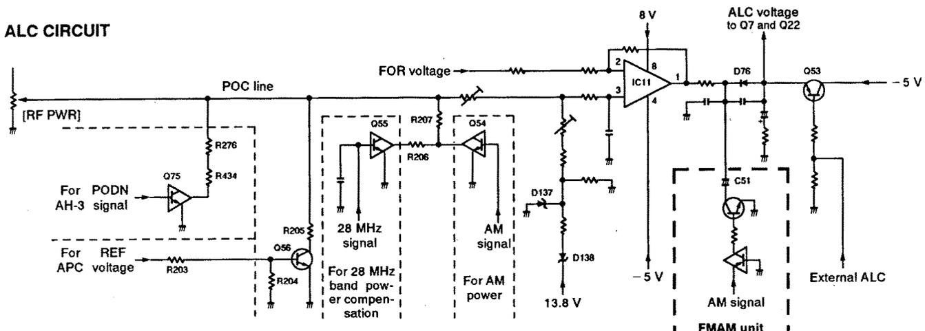
When the "REF" signal level increases, Q56 decreases the POC line voltage via R205. The POC line voltage is applied to IC11 to activate the ALC.
