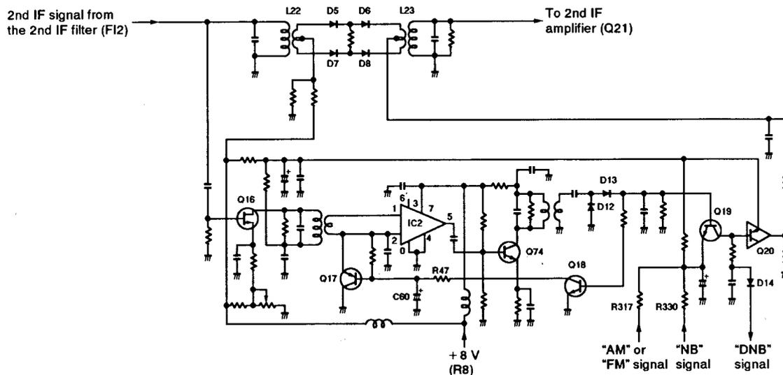
A portion of the detected signal from the noise detector is applied to the noise AGC circuit (Q17, Q18, C60, R43, R47) to control the bias voltage of the noise amplifier (IC2 pins 1, 2).
