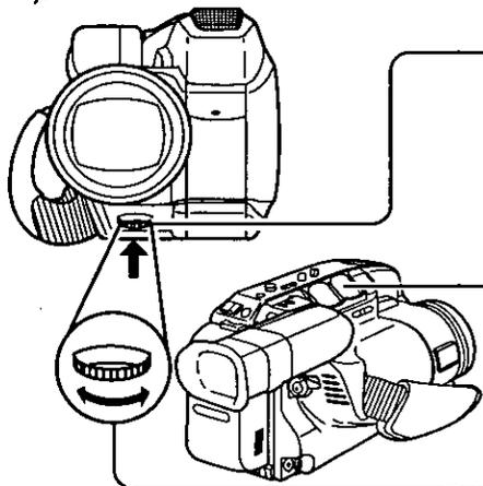
**1** Press **MANUAL FOCUS** so that "MF" (Manual Focus) appears in the EVF.
