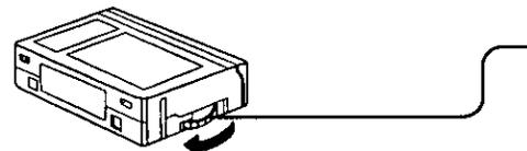
**1** Turn the Tape Wheel on the **VHS** cassette in the direction of the arrow to take up any slack.
