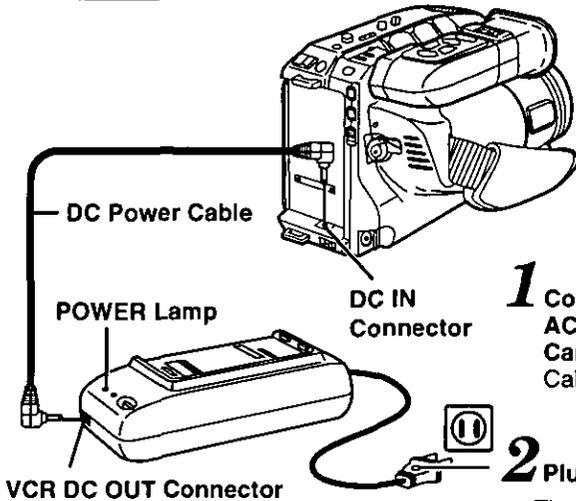
**1** Connect VCR DC OUT on the AC Adaptor to DC IN on the Camcorder with the DC Power Cable (supplied).
