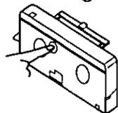
**2** Hold the PlayPak securely in one hand. Using your finger, reach through the hole in the bottom of the PlayPak Adaptor and push the tape out the top.
