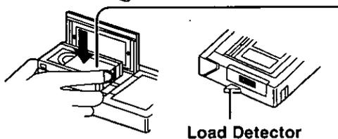
**3** Insert the **VHS** cassette with the window facing up and to the left. Then, snap the lid shut.
