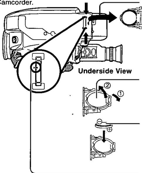
**1** While pinching the stopper tabs, pull the Battery Tray out of the Battery Compartment.
