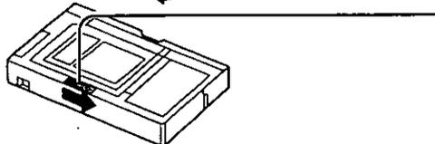
**2** Slide the **RELEASE** button in the direction of the arrow to open the PlayPak door.
