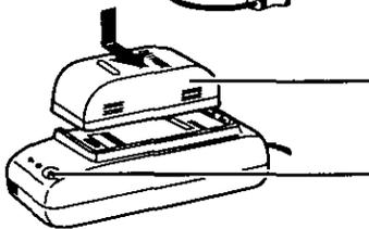
**2** Place the Battery into the AC Adaptor.
