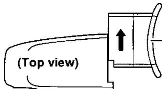
**2** Slide the eyepiece in the direction of the arrow. (DO NOT TWIST)
