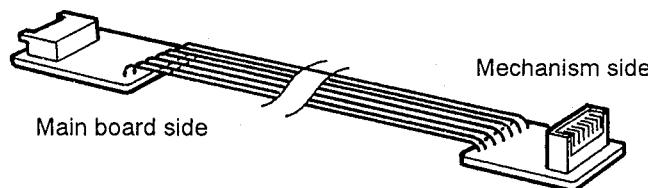
For connection between mechanism assembly and main board assembly.
