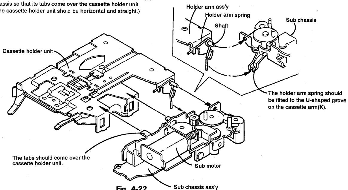
**Fig. 4-22****Step 4. Installing the cassette holder unit and sub chassis to the chassis.**
