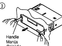
**When installing the unit without using the sleeve.**
