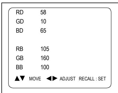
Using volume up or volume down, adjust service adjustment data of RD/GD/BD and RB/GB/BB until a good gray scale with normal whites is obtained.
