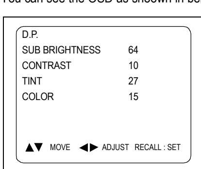
Select Subbrightness item, adjust Subbrightness data value to obtain normal brightness level.
