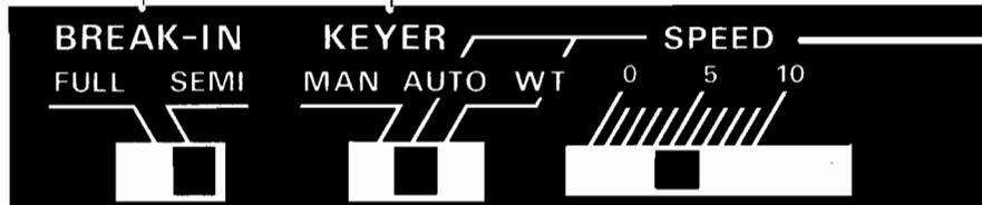
For CW operation (with or without the internal keyer) this switch selects the type of transmit/receive switching between code elements. Select the **FULL** position for full break-in (QSK), if you want the receiver to be activated between each dot and dash. Select the **SEMI** position if you want the receiver to be activated only when you pause while sending. Related adjustments are described on page 20.
