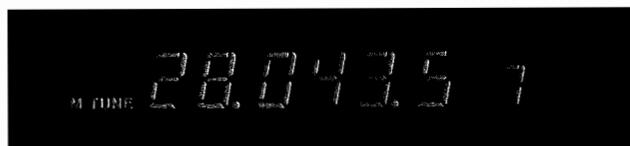
M TUNE mode display of retuned memory 18 (+10 Hz). Press **VFO/M** once to cancel changes and revert to MEM mode, and press it again to return to VFO mode.
