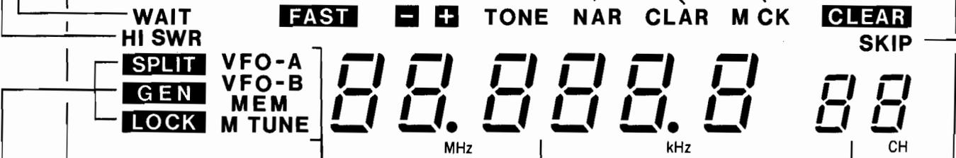
These three indicators appear when the respective functions are active: split transceiver (page 21), GENeral coverage (100-kHz) DOWN/UP stepping (page 13), and dial or panel lock (page 15).
