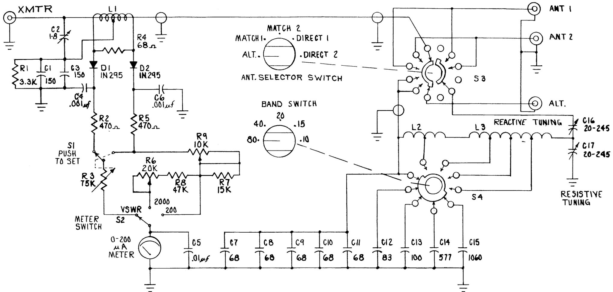
Figure 4-1. Model MN-2000 Matching Network Schematic Diagram
