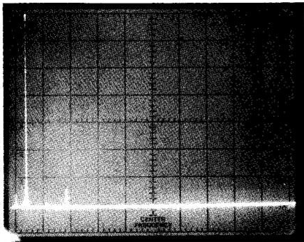
Fig 1—ICOM IC-765 worst-case spectral display. Horizontal divisions are 10 MHz; vertical divisions are 10 dB. Output power is approximately 121 W at 3.52 MHz. All harmonics and spurious emissions are at least 64 dB below peak fundamental output. The IC-765 complies with current FCC specifications for spectral purity for equipment in this power-output class and frequency range.
