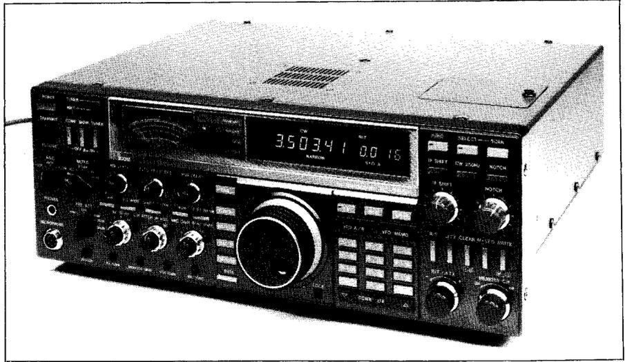
10 Hz (the '761's display resolved frequencies to the nearest 100 Hz). The display-calibration control, located on the front panel of the IC-761, is located under a panel on top of the IC-765. Unfortunately, ICOM didn't include a front-panel display-intensity control.
