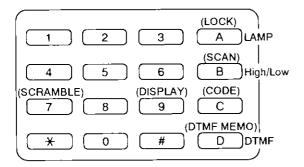
Except for DTMF codes (0–9,  $\frac{1}{2}$ , #, A–D), the keys on the keypad are not labelled. Use the diagram above as a quick reference for key functions during operation.
