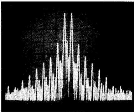
Fig 1—Spectral display of the TS-50S transmitter during two-tone intermodulation distortion (IMD) testing. Third-order products are approximately 30 dB below PEP output, and fifth-order products are approximately 42 dB down. Vertical divisions are 10 dB; horizontal divisions are 2 kHz. The transceiver was being operated at 100 W PEP output at 14.2 MHz.
