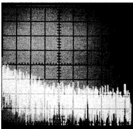
Fig 3—Spectral display of the TS-50S transmitter output during composite-noise testing. Power output is 100 W at 14 MHz. Vertical divisions are 10 dB; horizontal divisions are 2 kHz. The log reference level (the top horizontal line on the scale) represents  $-60$  dBc/Hz and the baseline is  $-140$  dBc/Hz. The carrier, off the left edge of the photograph, is not shown. This photograph shows composite transmitted noise from 2 to 20 kHz from the carrier.
