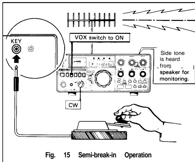
Fig. 15 Semi-break-in Operation
