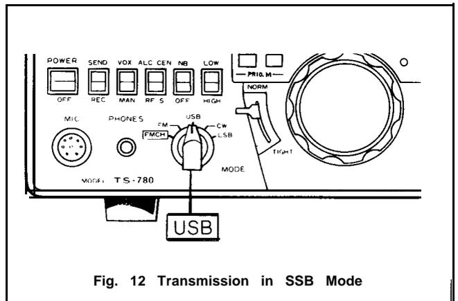
Fig. 12 Transmission in SSB Mode
