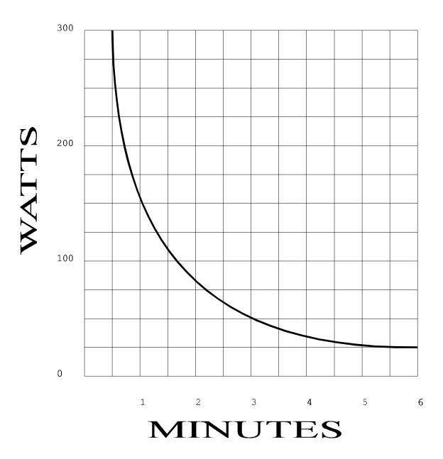
Derating curve for the MFJ260 Dummy Load.
